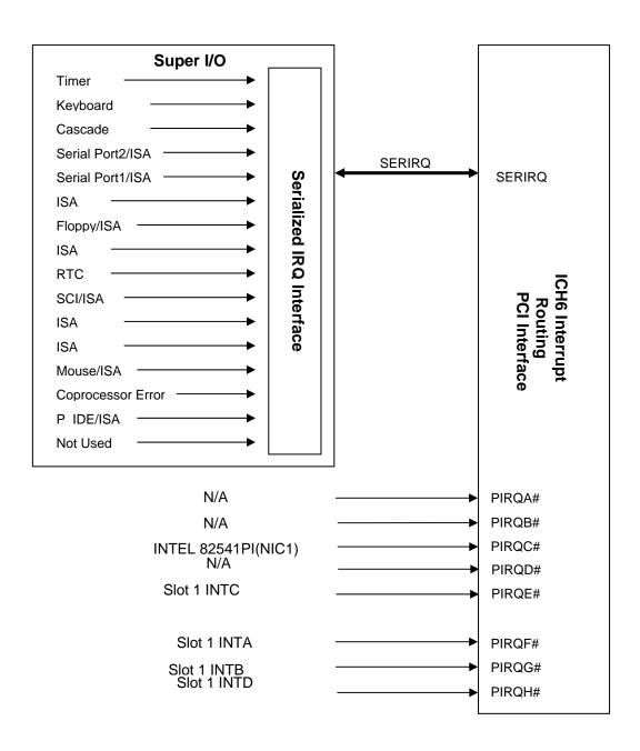
Figure 4. ICH6R Interrupt Routing Diagram
